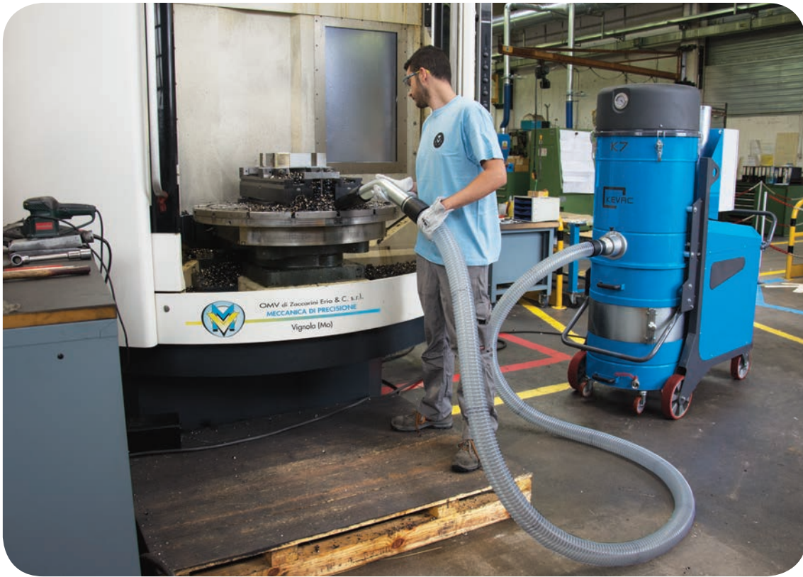
Swarf vacuuming onto a 5 axis universal machining centre
